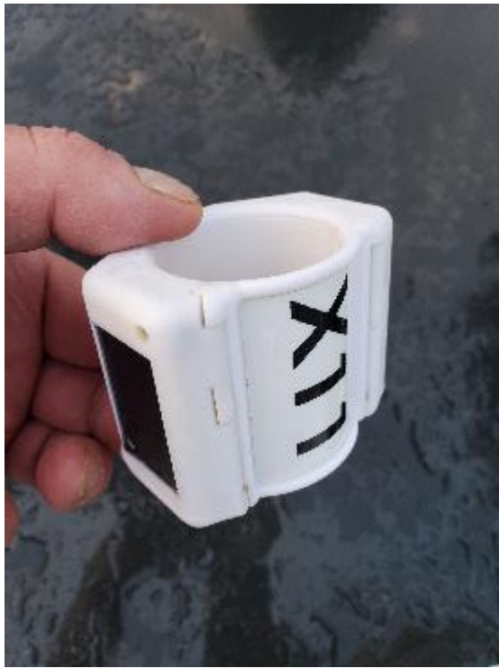
Satellite transmitter, mounted on neck collar, 3 solar panels
